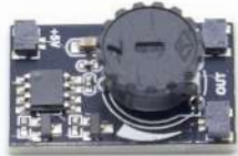
Dimmer Control Board
