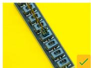
Not only will a light connected to the damaged port not work, but if the pins inside the port are bent to a point they are touching each other, this can result in all other lights in the system to stop working. This is a short circuit.
