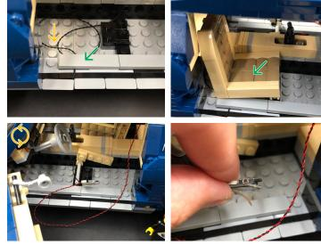
Ensure the NC push button is facing out and the edge of the board is in line with the edge of the door way, so that when the door closes, it pushes the button to de-activate the internal light.
