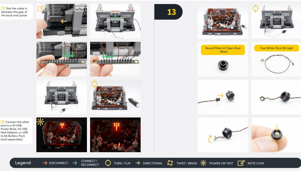
If you experience any issues with the lights not working and suspect an issue with a component, please try a different port on the expansion board to verify where the fault lies (with the light or
