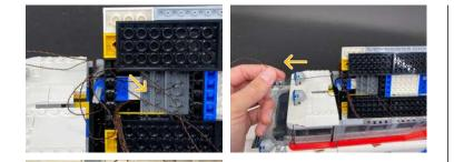
Ensure you connect the Bit Light to the 6-Port Expansion Board from step. 36 NOT from step. 35
