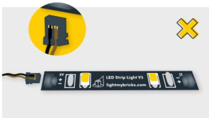
**CAUTION:** If plug won't fit easily into a port, don't force it. Doing so will damage the plug and the port.
